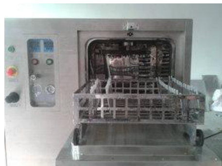
Cleaning room(Stainless steel304)
